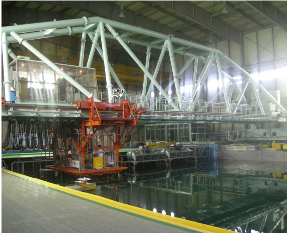
Fig. 2: Computerized Planar Motion Carriage(CPMC) of MOERI.
