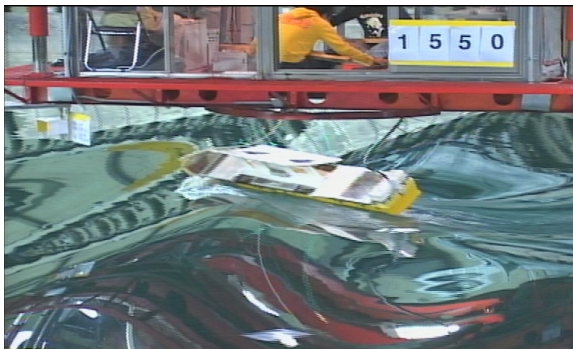
Fig. 6: Photograph of Large Roll Motion in Quartering Sea (GM=1.2m, \lambda=1.5L_{pp} , Vs=25kts, \chi=15\text{deg} , H/ \lambda=1/18 )
