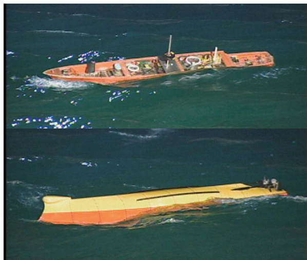
Figure 1. View of Model 5514 During Capsizing Testing In MASK Basin.
