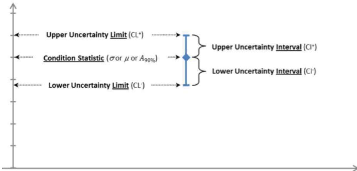
**Fig. 4** Metric Nomenclature (condition statistic, interval, and limit)
