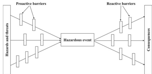
Figure 3: Simplified bowtie diagram [5]
