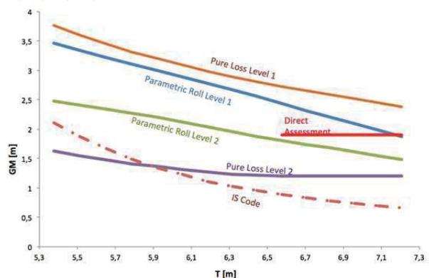
Figure 9 : GM<sub>Req</sub> curves for the RoPax 1
