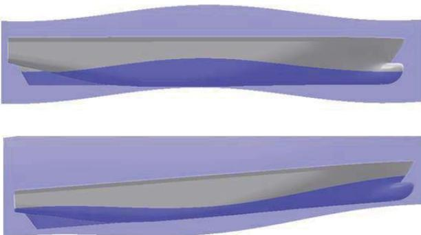
Figure 1: Wave with the length of the ship with crest and trough located at amidships.
