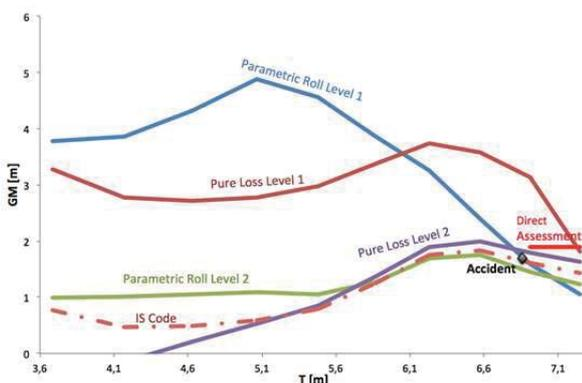
Figure 14: GM required curves for the RoPax 4
