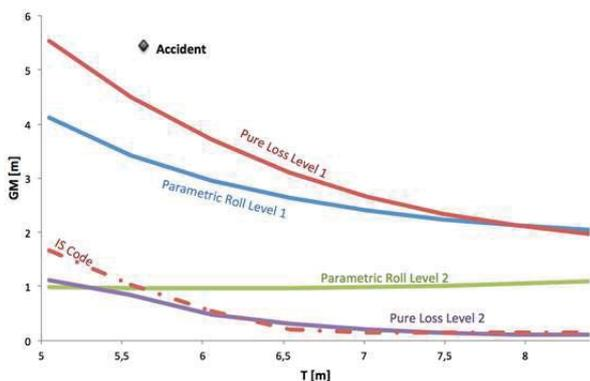
Figure 17: GM required curves for the Container 3
