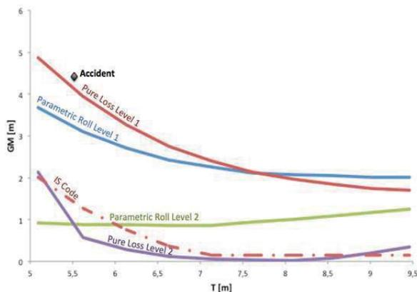
Figure 16: GM required curves for the Container 2
