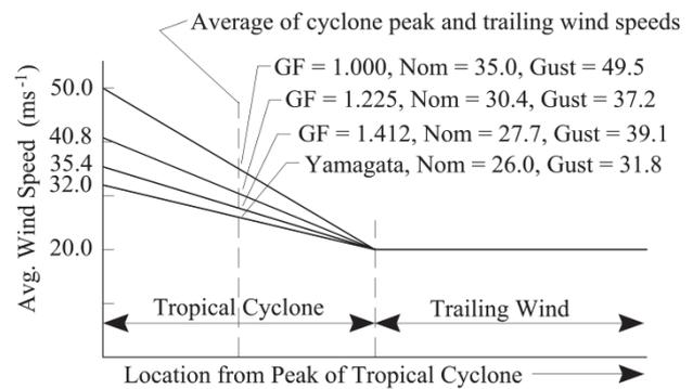
Figure 4 Simplified typhoon wind velocity, adapted from Yamagata (1959)
