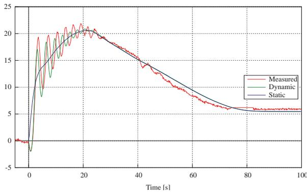
Figure 6 Case A: Roll motion measured and computed
