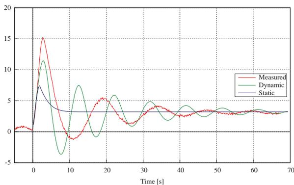
Figure 9 Case B: Roll motion measured and computed
