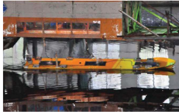
Fig.6 The ship model in free decay test
