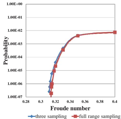
Figure 11 Effect of calm-water resistance modelling on surf-riding probability of the PCC
