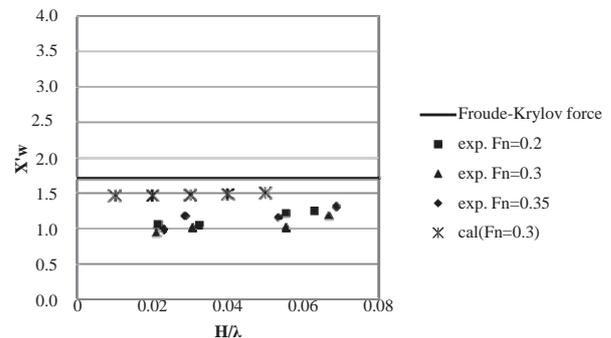
Figure 1 Wave-induced surge force for the ITTC A1 containership with the wavelength to ship length ratio of 1 for different wave steepnesses,  $H/\lambda$ , and the Froude numbers,  $F_n$ . Here the wave-induced surge force is normalized with the product of ship weight and wave steepness. (Y. Ito, et al., 2014).
