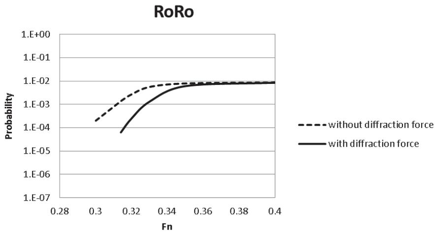
Figure 4 Surf-riding probability for a RoRo ship with and without diffraction effect.
