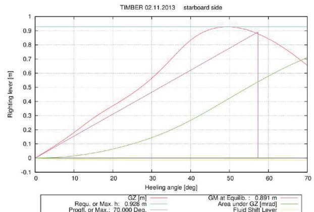
Figure 5 Lever arm curve during the departure time
