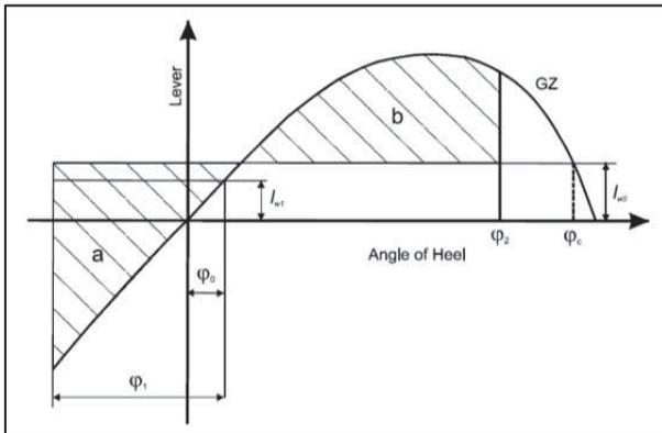
Figure 2 Graphical representation of the weather criterion
