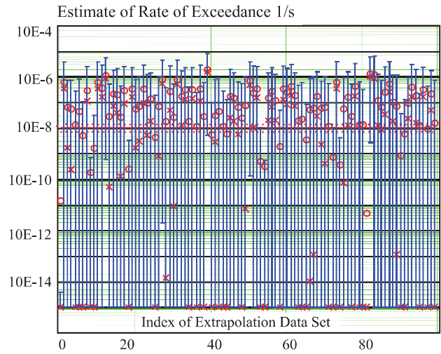
Figure 5 Confidence interval overlap of true value for lateral acceleration at 45 deg heading at 0.3g comparison level using logarithm CI
