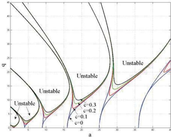
Fig.1 Stability chart of single-frequency excitation
