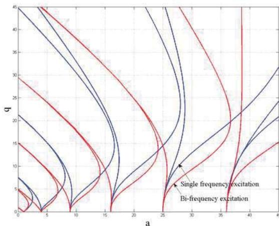
Fig.3 Stability chart for single- and bi-frequency excitation ( $d=-0.5$ )
