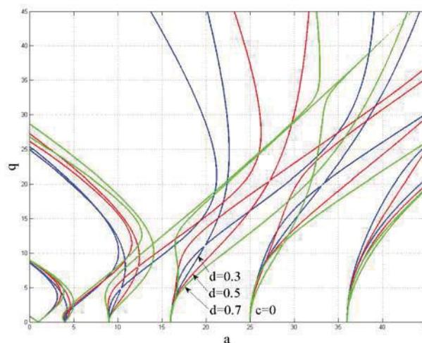
Fig.9 Stability chart for bi-frequency excitation for different d ( $c=0.0$ )
