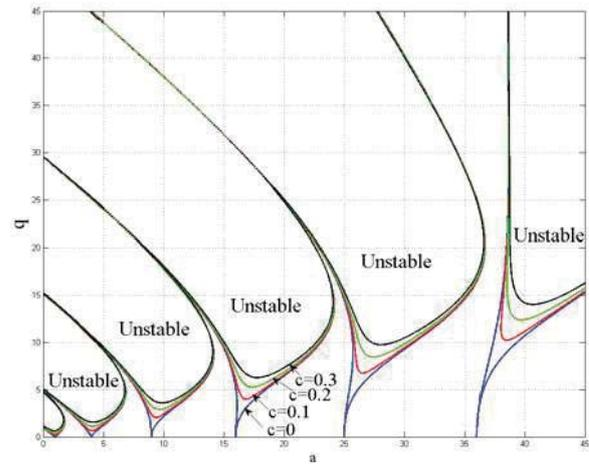
Fig.4 Stability chart for bi-frequency excitation for different damping ( $d=-0.5$ )
