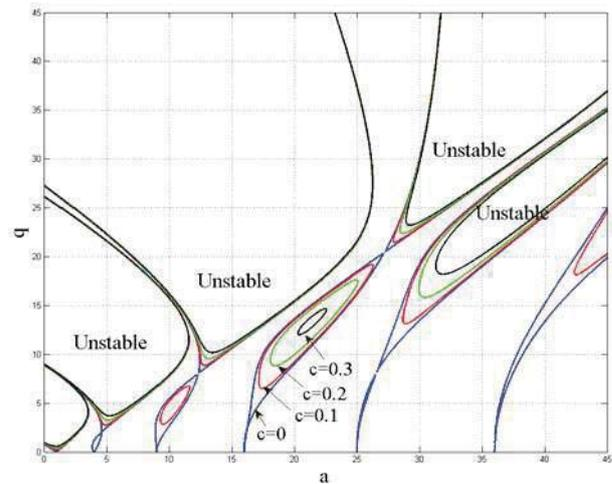
Fig.5 Stability chart for bi-frequency excitation for different damping ( $d=0.5$ )
