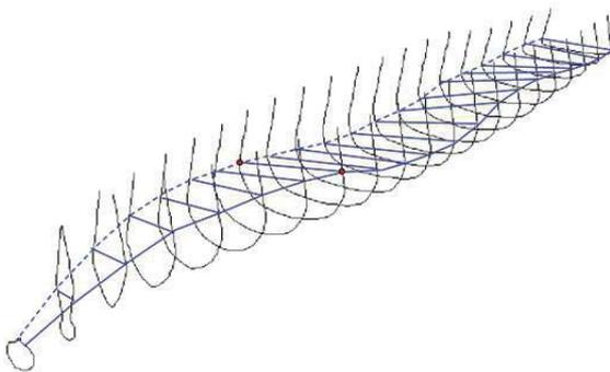
Figure 2: Station/incident wave intersection points for the ONR Tumblehome hull in stern oblique seas
