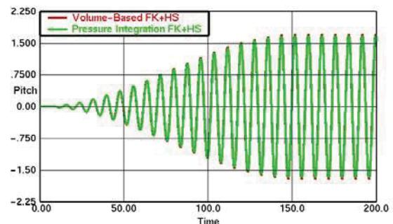
Figure 6: Pitch motion for rectangular barge in quartering regular waves,  $\lambda=L$   $h=d/3$
