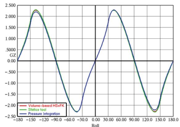
Figure 3: Calm water restoring curve for rectangular barge
