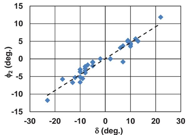
Figure 3 Measured heel angles and rudder angles in the experiment.
