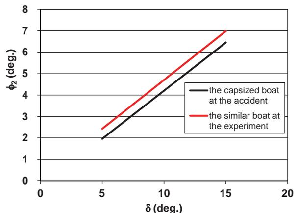
Figure 7 Outward heel angle due to steering.
