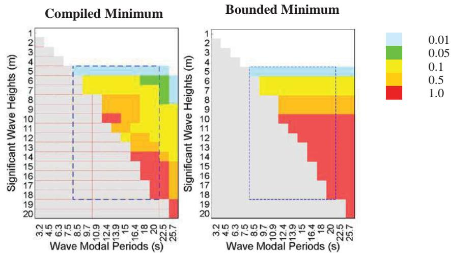
Figure 15. Minimum ranges of Wave Height and Period.
