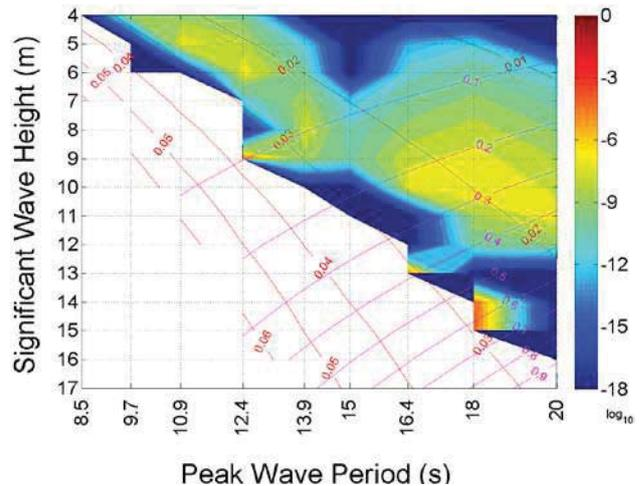
Figure 19. O(MPECRA-VB) by Wave Height and Period in Phase 2 Load Condition 6 (Phase 3 Equivalent Range of Height and Period).
