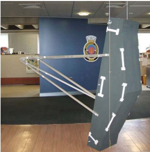
Figure 4 Establishing KG by suspension
