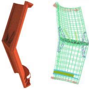
Figure 2. 3D model of V-form trawling board for combination the centre of elastic forces («the centre of shear») with centre of gravity.
