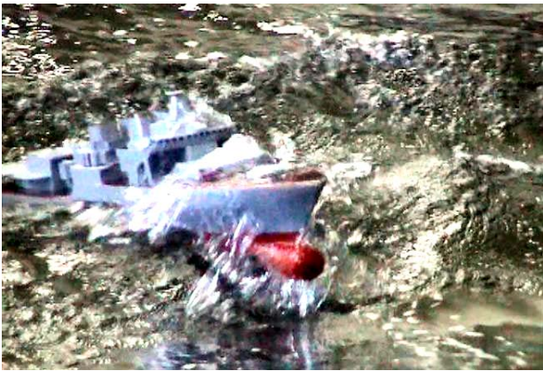
Figure 5. Inadmissible that overweening speed on bow seas was subjected to the ship. It means that ship design instead of undersea bulbous and spreading bilge, must be use a tumblehome stem with trimming underwater peak, and small volume in bow freeboard.
