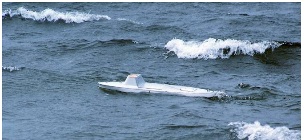
Figure 7. Maritime experiment with optimized hull form for model of ship on stormy sailing under intensive influence from breaking waves on shallow water.
