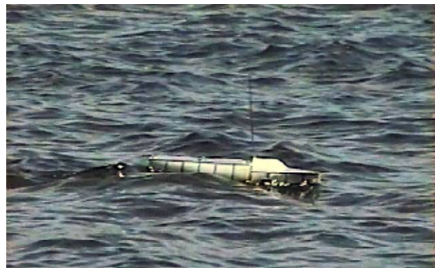
Figure 10. Almost fully transformation pitching to heaving of ship was reached in this design of a small remote control vehicle with flapping wing propulsion. Experimental test was confirmed propulsive quality and small pitching of ship on intensive waves sailing.
