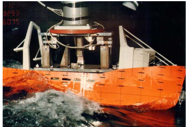
Figure 2. Fully captive model tests in waves (Grochowalski, 1989).
