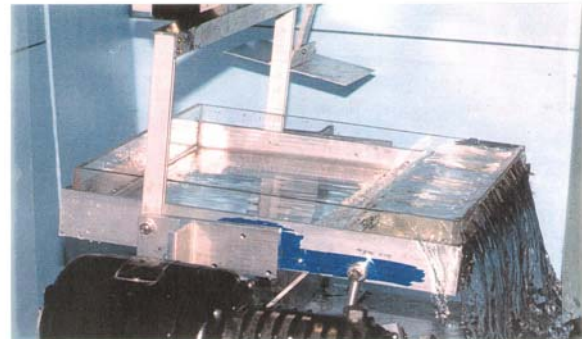
Fig. 4-2 Water Escaping off the Deck (Waterfall)
