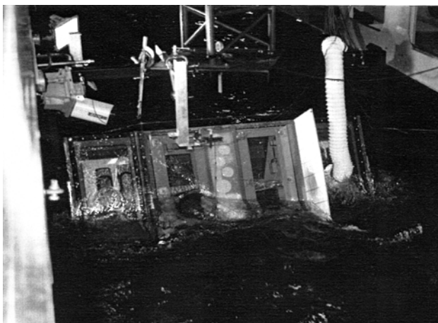
Figure 12. Investigation of hydrodynamic forces on submerged part of deck (Grochowalski, 1997).
