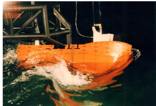
Figure 4. Partly captive model tests in waves. The model is free to heave and pitch (Grochowalski, 1989).
