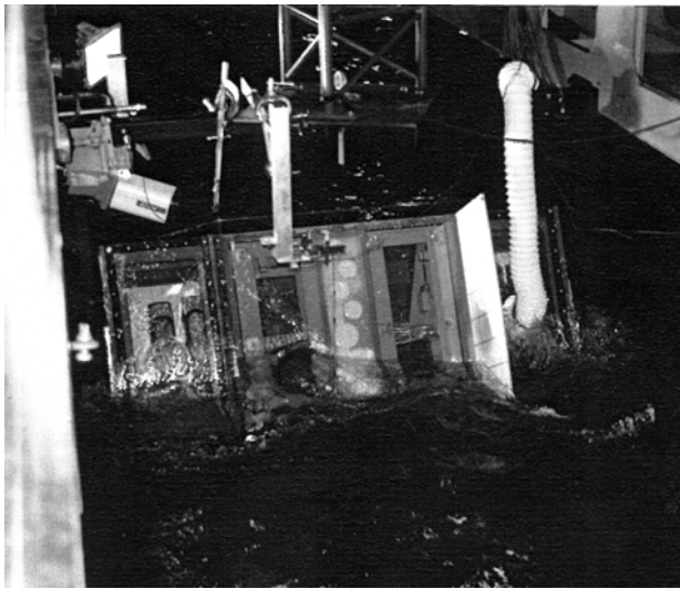
Figure 3. Experiment setup for deck-in-water testing.
