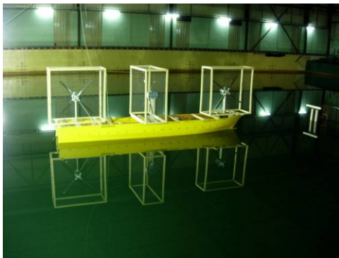
Figure 5. Model fitted with fans for wind force simulation.
