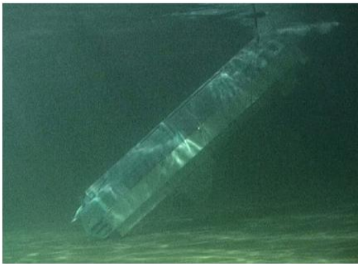
Figure 11. Model test in MDL. After capsizing the ship sank with stern first.
