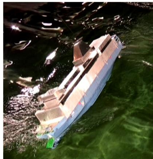
Figure 10. Model test in MDL. When the bow visor was lost and the ramp was open, a large amount of water was entering the car deck resulting in a rapidly growing starboard list.
