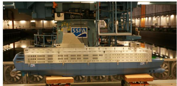
Figure 9. The scale model of MV Estonia . In the background SSPA's Maritime Dynamics Laboratory (MDL) is shown.
