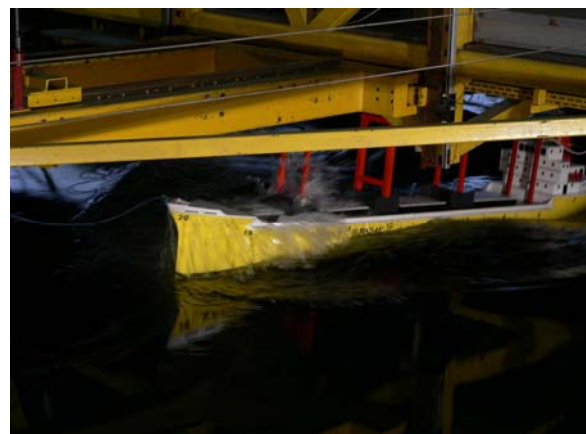
Figure 2. Illustration of intensive deck wetness at head seas.
