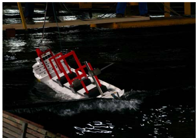
Figure 7a. Final phase of surf-riding – large wave is passing along the ship, water is pouring into an opening in the hold.
