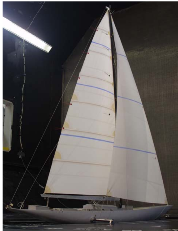
Figure 6. Model used for maximum heeling moment tests.
