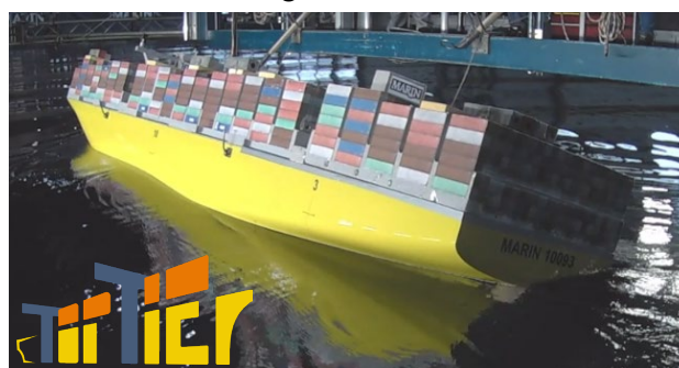
Figure 2: Example of parametric roll in following seas for a 10,000 TEU container vessel (wave height 4 m, wave period 11.9 s, vessel speed 10.6 kn, max. roll angle 19.7 deg)
