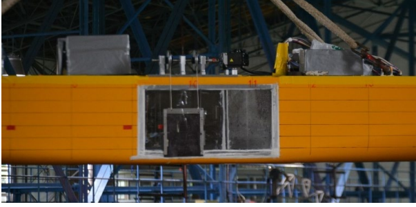
Figure 3: Self-designed electrically operated valve for controlling the opening's size.
