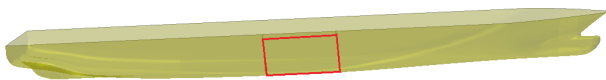
Figure 1: The geometry of the damaged hull (the position of the damaged cabin is marked in red)
