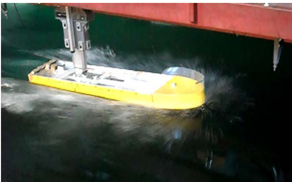
Figure 2: UNINA model experimental set up (photo at model speed V = 5.75\text{m/s} ).
