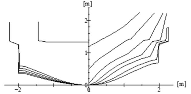
Figure 2: Body plan of the target ship.
