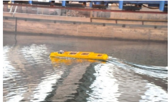
Figure 2: A snapshot of surf-riding in the free running experiment
