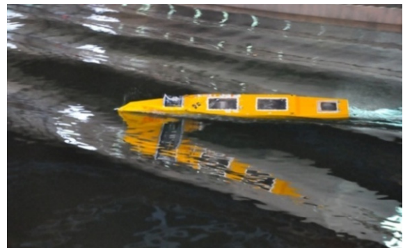
Figure 3: A snapshot of broaching in the free running experiment
