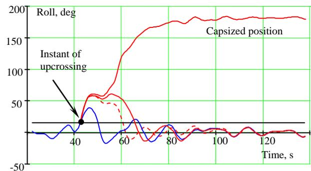
**Figure 2: Calculation of critical roll rate (Belenky, et al. 2016b)**
