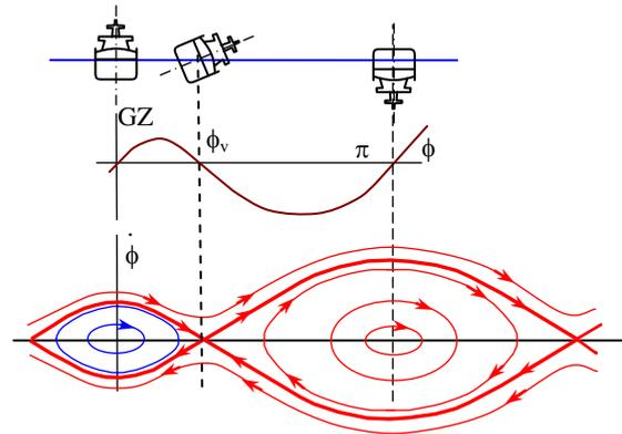
**Figure 1: Phase plane of un-damped roll motion.**
