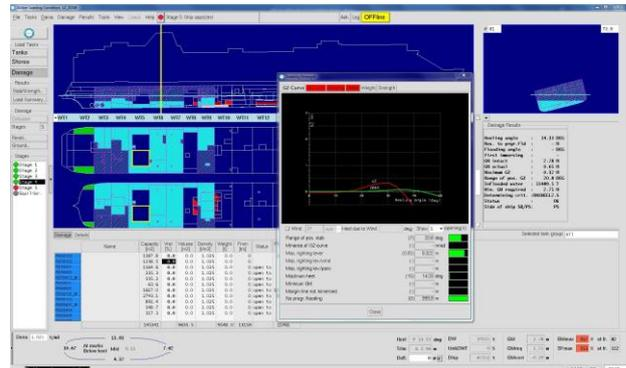
Figure 4: Example of damage stability results from a loading computer
