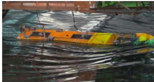
**Figure 4: The 4250TEU containership model in the free running experiment.**
