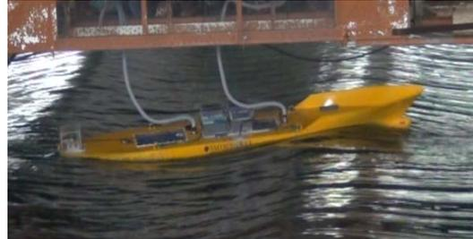
**Figure 3: The passenger ship model in the free running experiment.**
