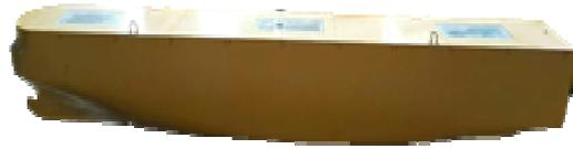
**Figure 2: The pure car carrier model in the free running experiment.**
