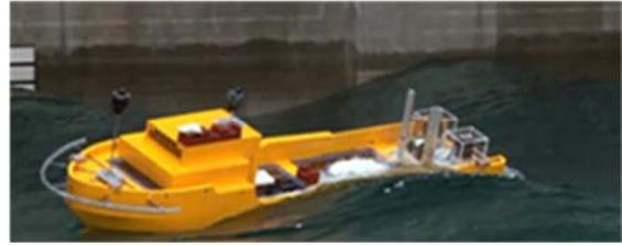
Fig.2 Free-running model experiment of the OSV in stern quartering waves
