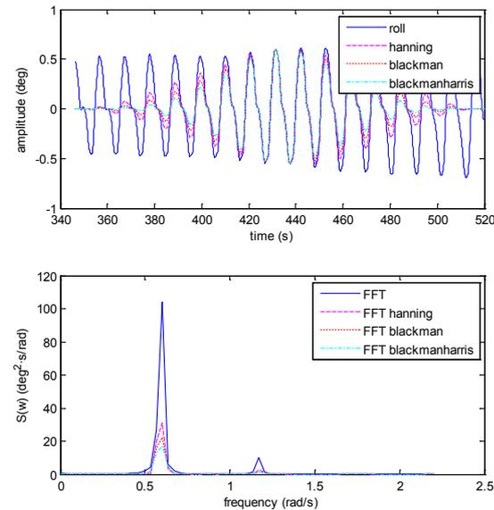
Figure 4. Test 2. Regular waves. Fn 0. No parametric roll.
