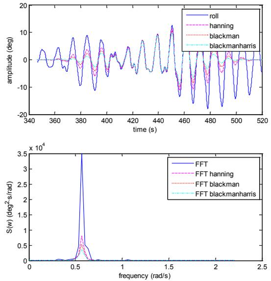
Figure 5. Test 3. Irregular waves Fn 0. Parametric roll occurs.
