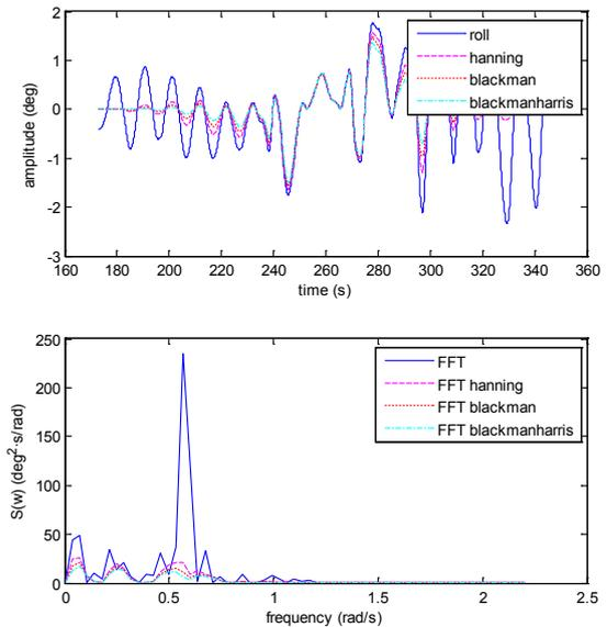
Figure 6. Test 4. Irregular waves. Fn 0.1. No parametric roll.
