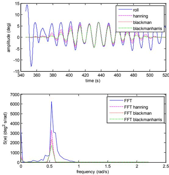
Figure 3. Test 1. Regular waves. Fn 0.1. Parametric roll occurs.
