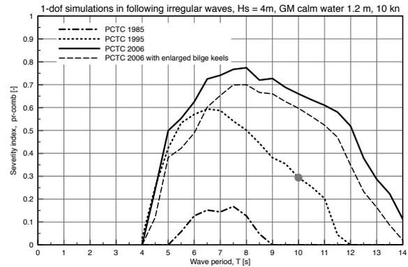
**Figure 4:** Qualitative comparison of different PCTC generations with regard to parametric roll. Results from 1-dof simulations in following waves with  $H_s$  4m and varying wave periods. The effect of enlarged bilge keels on the most sensitive ship type is also included. The dot represents the simulated sequence in Figure 3 and the condition is similar to the real case shown in Figure 1.
