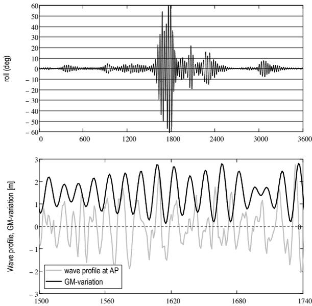
**Figure 3:** Example of results from a simplified 1-dof simulation of parametric rolling in following irregular sea. The upper graph shows a 1h roll sequence with typical parametric rolling. The lower graph shows a small sequence of four minutes with wave profile and  $GM$  variation during the development of large amplitude rolling.
