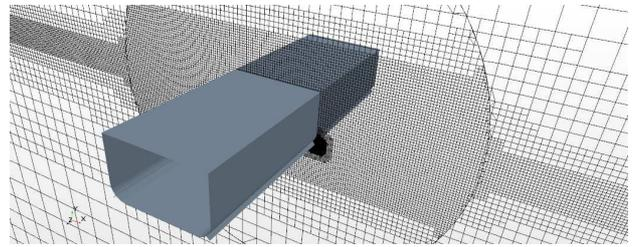
**Figure 1: The geometry and computational mesh**
