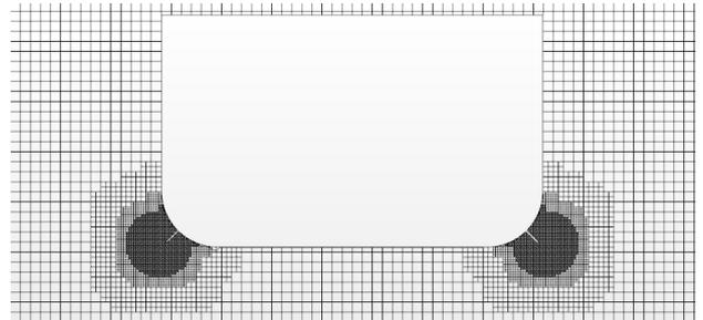
**Figure 2: The generated mesh around the hull and bilge keels**
