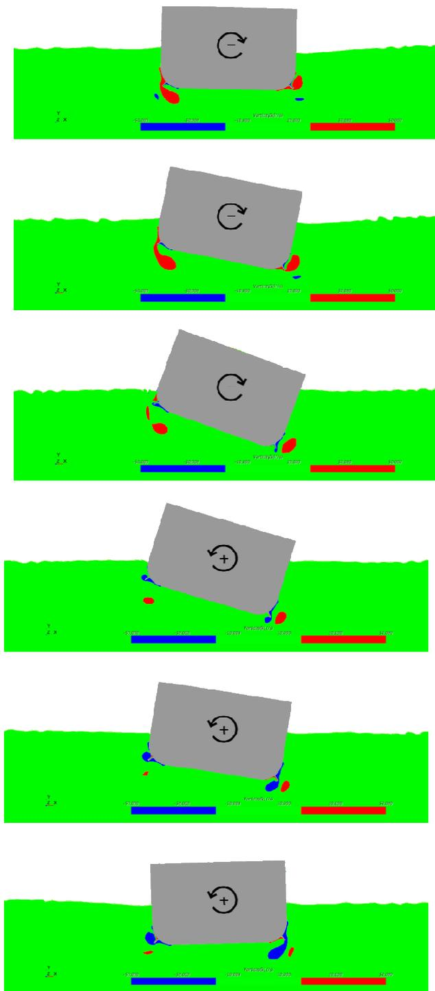
Figure 7: Vorticity contours and vortex shedding around the hull for 20.0 deg. roll amplitude
