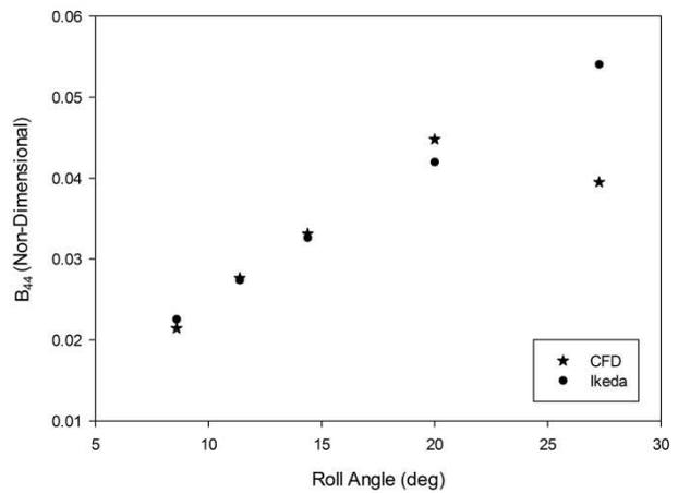
**Figure 5: Roll damping coefficients at different roll angles**
