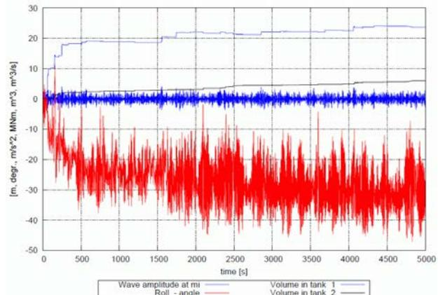
**Figure 1: Time plot of roll angle, wave elevation and floodwater ingress into two compartment during the sinking of the ORTEGAL UNO (BSU 14/10), see also Fig. 4, right.**
