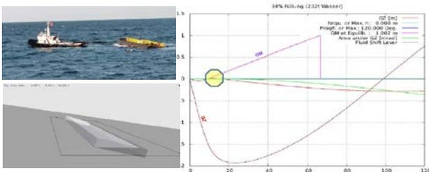
**Figure 3: Capsizing of a pontoon due to slow water ingress. (BSU 266/14). Left: Situation immediately before the capsize, right: Righting levers in that situation, free movement of the floodwater. Source: BSU**
