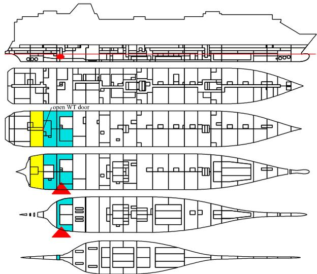
**Figure 3: Damage scenario, with initially open WT door that is closed before flooding progresses to the undamaged compartment**
