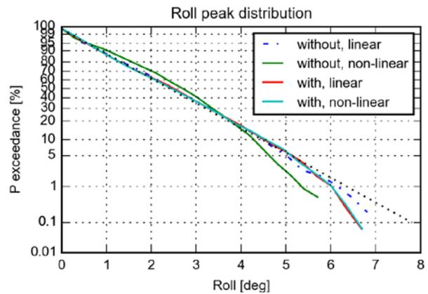
**Figure 12: Roll distribution, 1DoF time domain, Hs=0.5m, Tp=8.7s, with and without ART**
