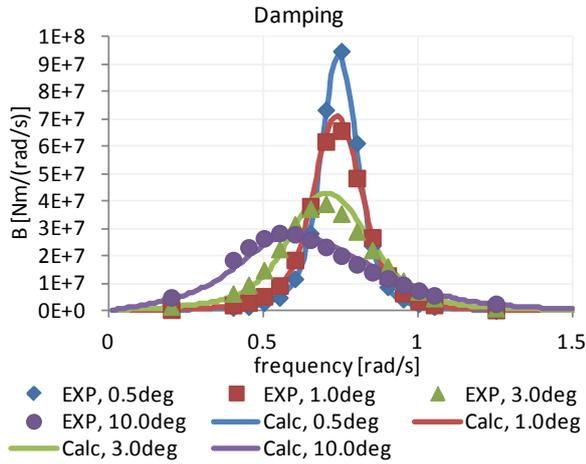
Figure 4: Damping of U-tank using Stigter's model
