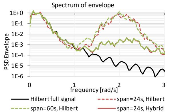
Figure 8: Spectrum of the envelope with various time spans
