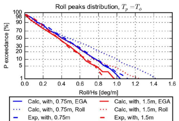
**Figure 15: Roll distribution, with tank, roll vs. EGA**
