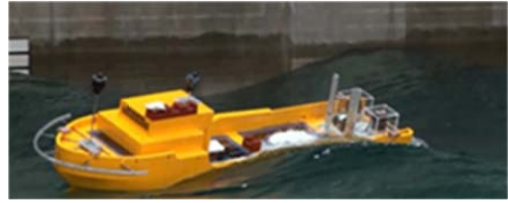
Fig.2 Free-running model experiment of the OSV in stern quartering waves
