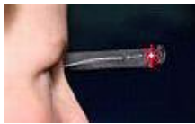
Figure 3. Peripheral detection task (PDT) for measuring workload.
