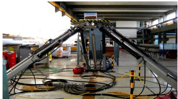
Fig.1: The shaking table equipment of NTUA's School of Naval Architecture and Marine Engineering.
