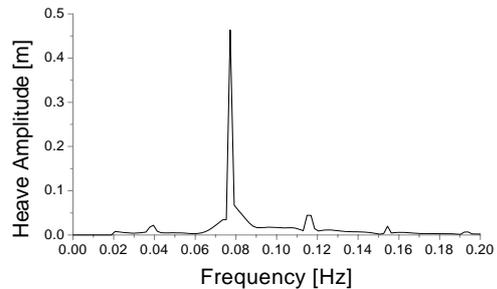
Fig.8 Parametric rolling, pitch and heave motions in time and frequency domains when the amplitude of parametric rolling is 25degs with  $\lambda/L_{pp}=1.0, H/\lambda=0.02, \chi=180^0, Fn=0.0, 1/(Te)=0.0772\text{HZ}$ . (Simulation)
