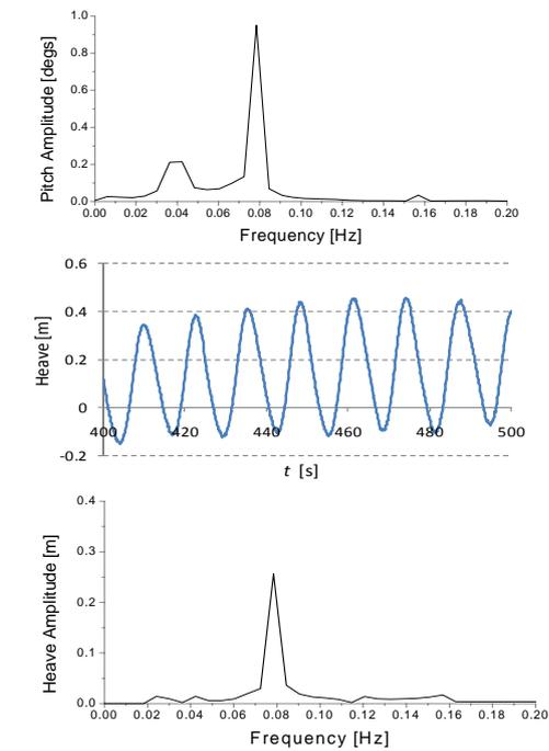
Fig.4 Pitch and heave motions in time and frequency domains when parametric rolling occurs with  $\lambda/L_{pp}=1.0$ ,  $H/\lambda=0.01$ ,  $\chi=180^\circ$ ,  $F_n=0.0$ ,  $1/(T_e)=0.0772\text{HZ}$ .
