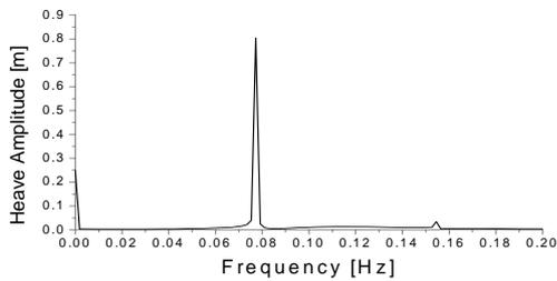
Fig.7 Pitch and heave motions in time and frequency domains without parametric rolling with  $\lambda/L_{pp}=1.0, H/\lambda=0.02, \chi=180^0, Fn=0.0, 1/(Te)=0.0772\text{HZ}$ . (Simulation)
