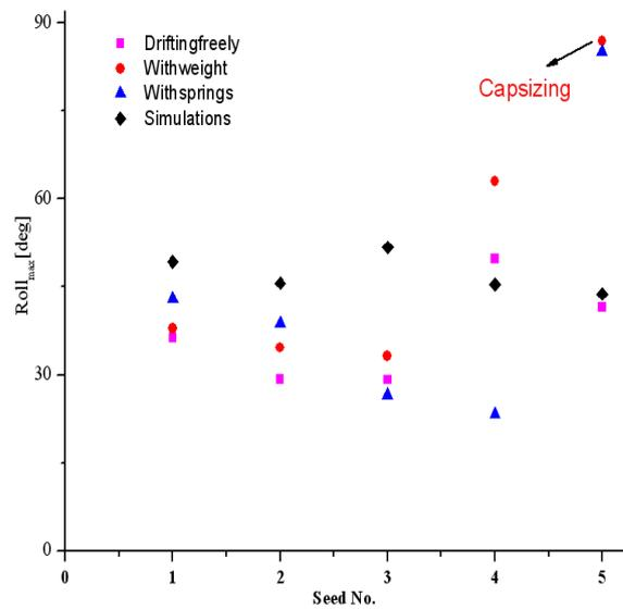
Fig. 7: Maximum roll angles in experiments and simulations with  $H_{1/3}=14.0m, T_{01}=12.38s, Fn=0.0, \chi=90^0, GM=1.781m$  and different seed numbers.
