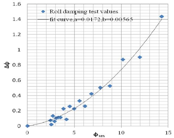
Fig. 4: Roll damping curves and Extinction curve (a, b are linear and square extinction coefficient).
