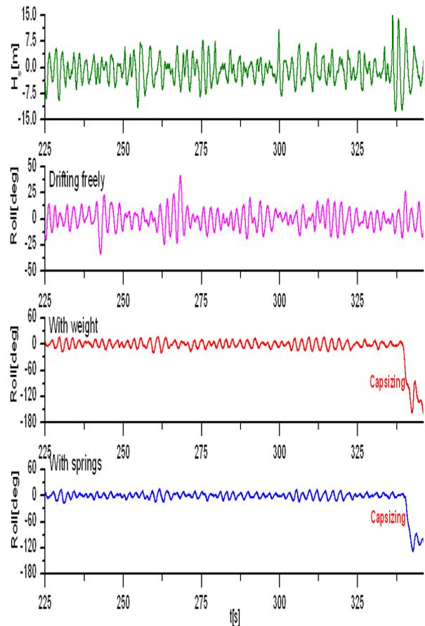
Fig.8: Wave profile and roll in time series with  $H_{1/3}=14.0, T_{01}=12.38, Fn=0.0, \chi=90^0, GM=1.781m$  and seeds number 5.
