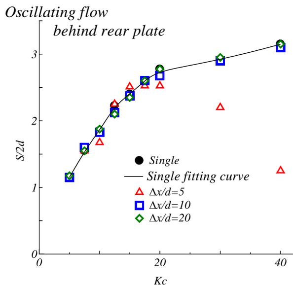
Fig.17 Vortex length at behind rear plate in oscillating flow
