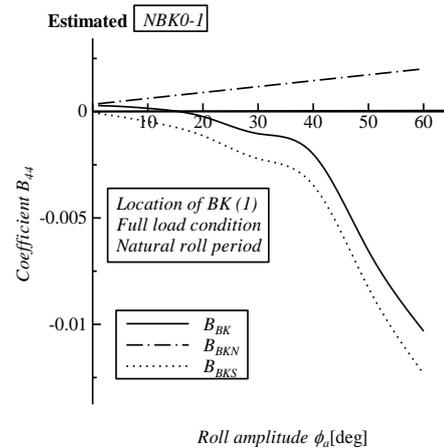
Fig.11 Total, normal-force and surface-pressure components of roll damping created by bilge keels predicted by Ikeda's method
