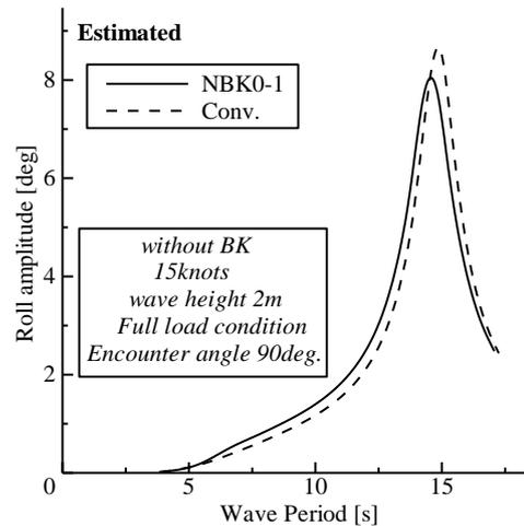
Fig.7 Estimated roll motions of ships without bilge keel at advanced speed
