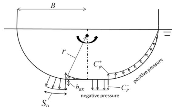
Fig.10 Assumed pressure distribution created by bilge keels in Ikeda's prediction method
