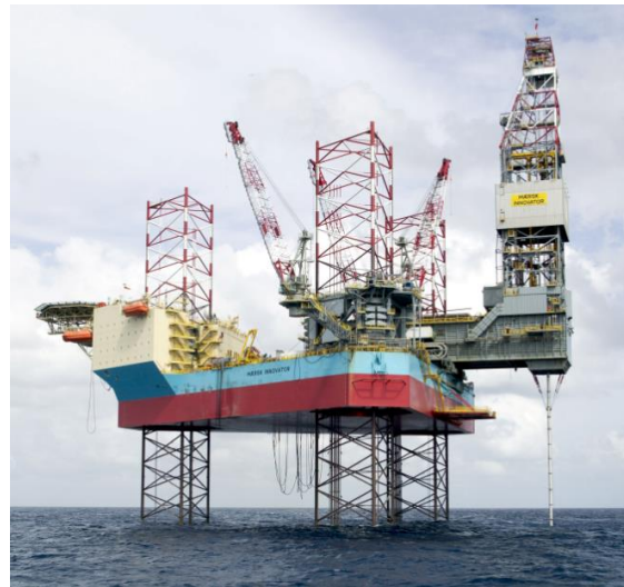
Fig. 3: Example of a large jack-up.
