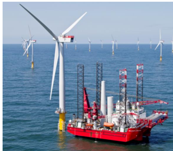
Fig. 4: Example of a small jack-up.
