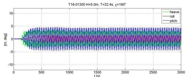
Fig. 3: Config. #1, regular wave, low wave amplitude, non-parametric resonant pitch
