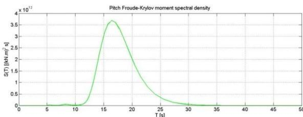
Fig. 20: Pitch Froude-Krylov moment spectral density,  $T=16,5s$ ;  $H=10m$ .
