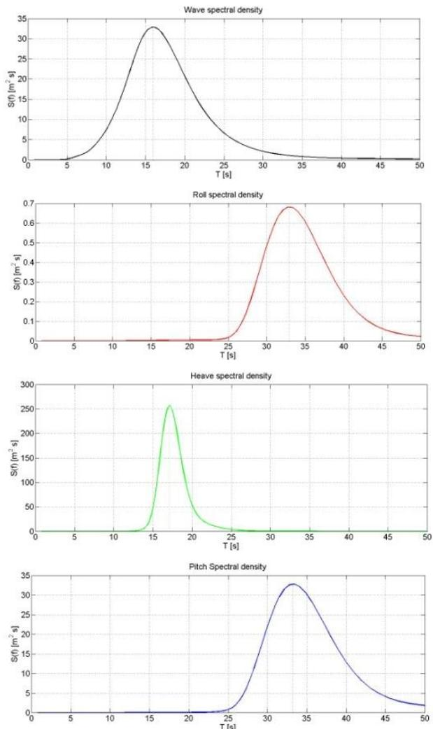
Fig. 11: Config #1, irregular waves, T=16,5s; Hs=5m. Wave, heave, roll and pitch spectra
