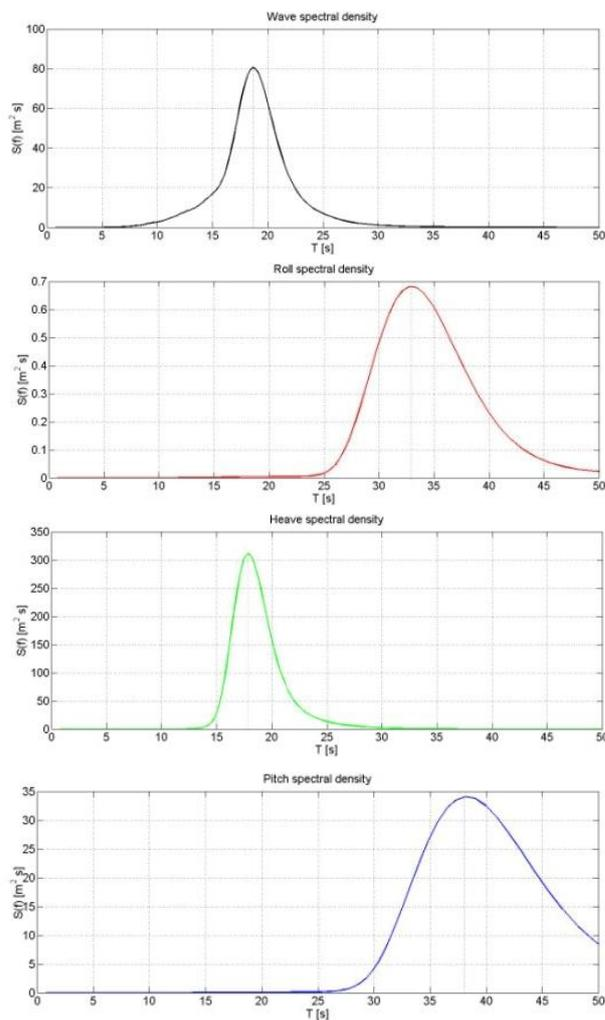
Fig. 15: T02200, Irregular waves, Config #3, T=18,9s; H=10m. Wave, heave, roll and pitch spectra
