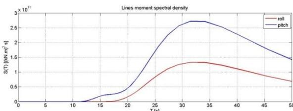
Fig. 22: Lines resultant moment spectral density,  $T=16,5s$ ;  $H=10m$ .
