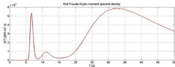
Fig. 21: Roll Froude-Krylov moment spectral density,  $T=16,5s$ ;  $H=10m$ .
