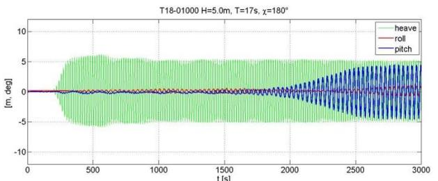
Fig. 4: Config. #1, regular wave, low wave amplitude, parametric pitch excited
