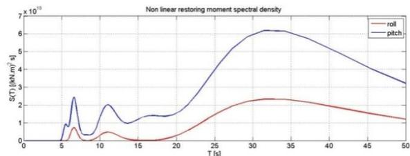
Fig. 19: Nonlinear restoring moment spectral density, T=16,5s; H=10m.
