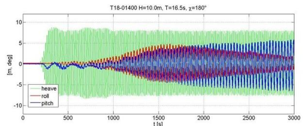
Fig. 5: Config. #1, regular wave, intermediate wave amplitude, roll and pitch are parametrically excited
