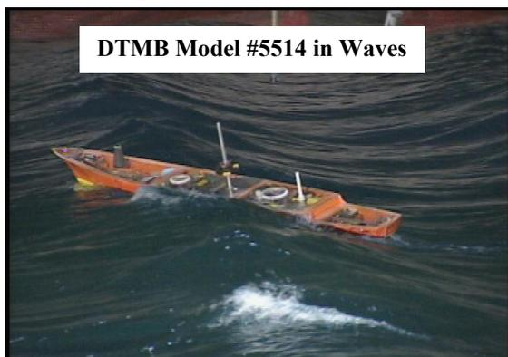
**Fig. 1. Experimental testing of ship performance in heavy seas using regular waves**
