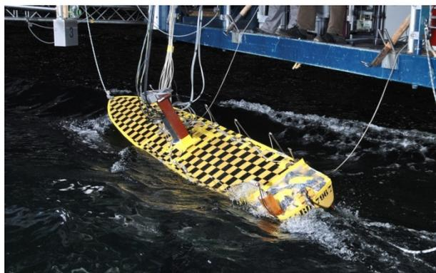
Fig. 2: High roll motion without capsizing and very low amount of green water in stern quartering seas.
