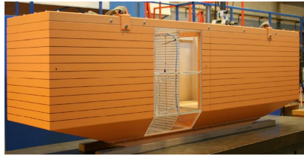
Fig. 1: Damage case arrangement
